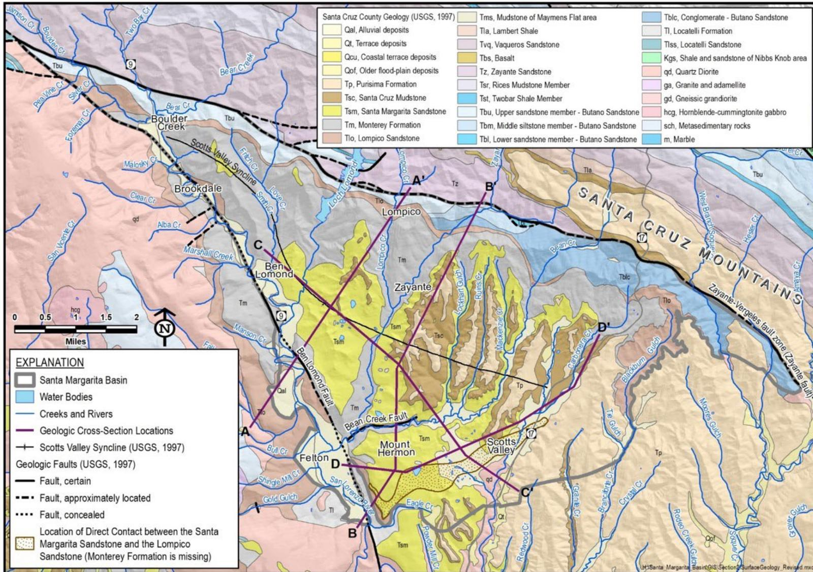
Figure 2. Surface Geology and Geologic Cross Section Locations
